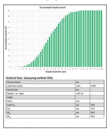
DV50 = MVD (Median volumetric diameter) = VMD (volume median diameter)
