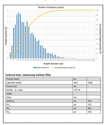
MND = NMD (number median diameter). Half of the droplet quantity is smaller, half is bigger than 19  $\mu$ m.
